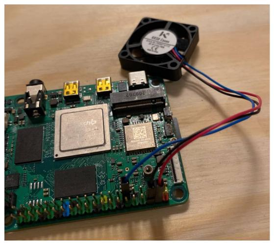
Connect Red to pin 4 Connect Black to pin 6 Connect Blue to pin 11
