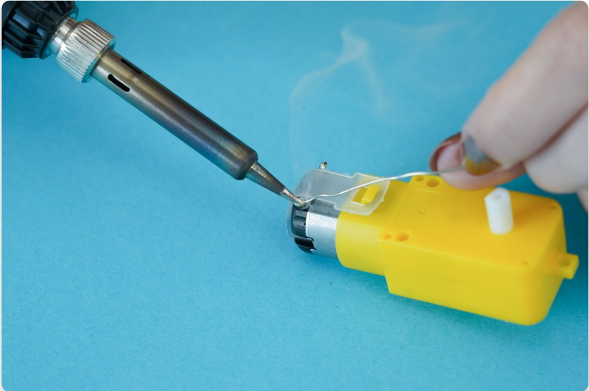
Put a generous amount of solder into the hole
