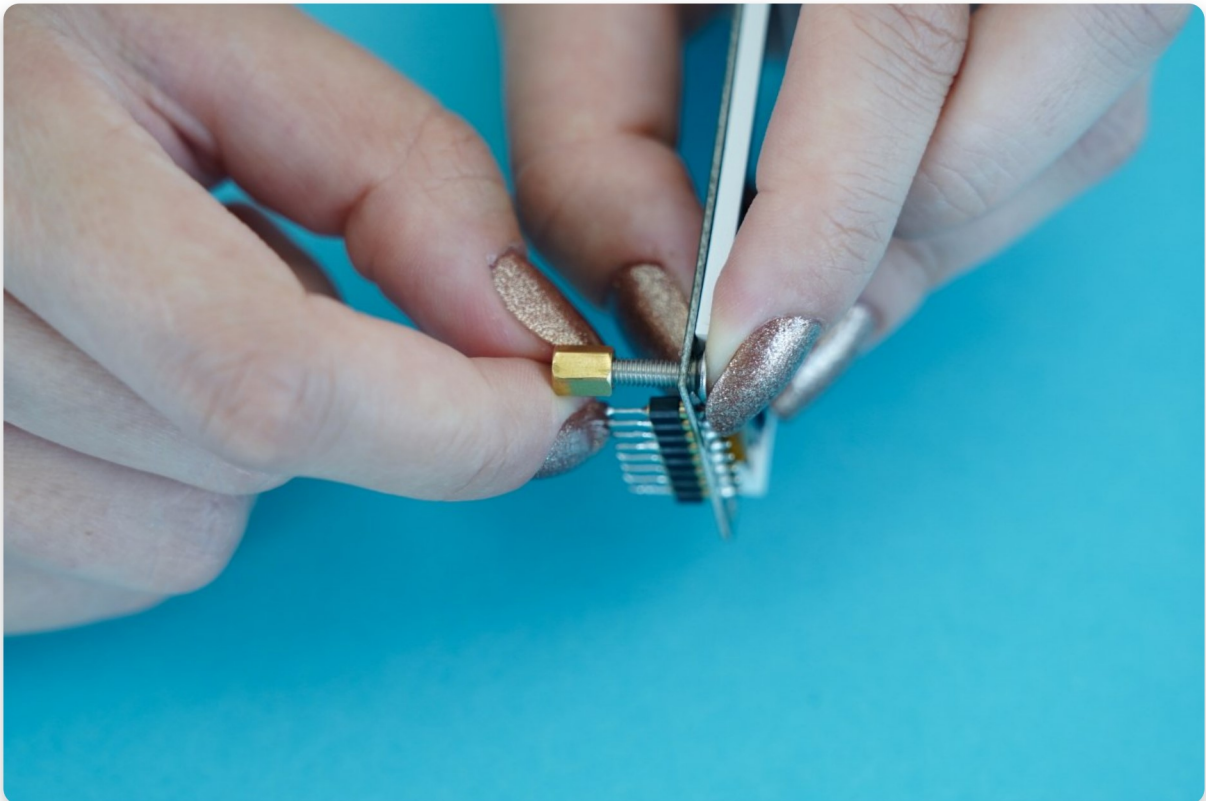
Twist on the brass spacer onto the end of the metal bolt
