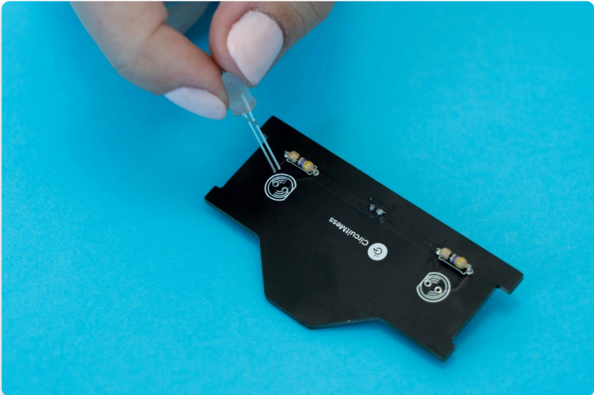
Insert the LEDs
