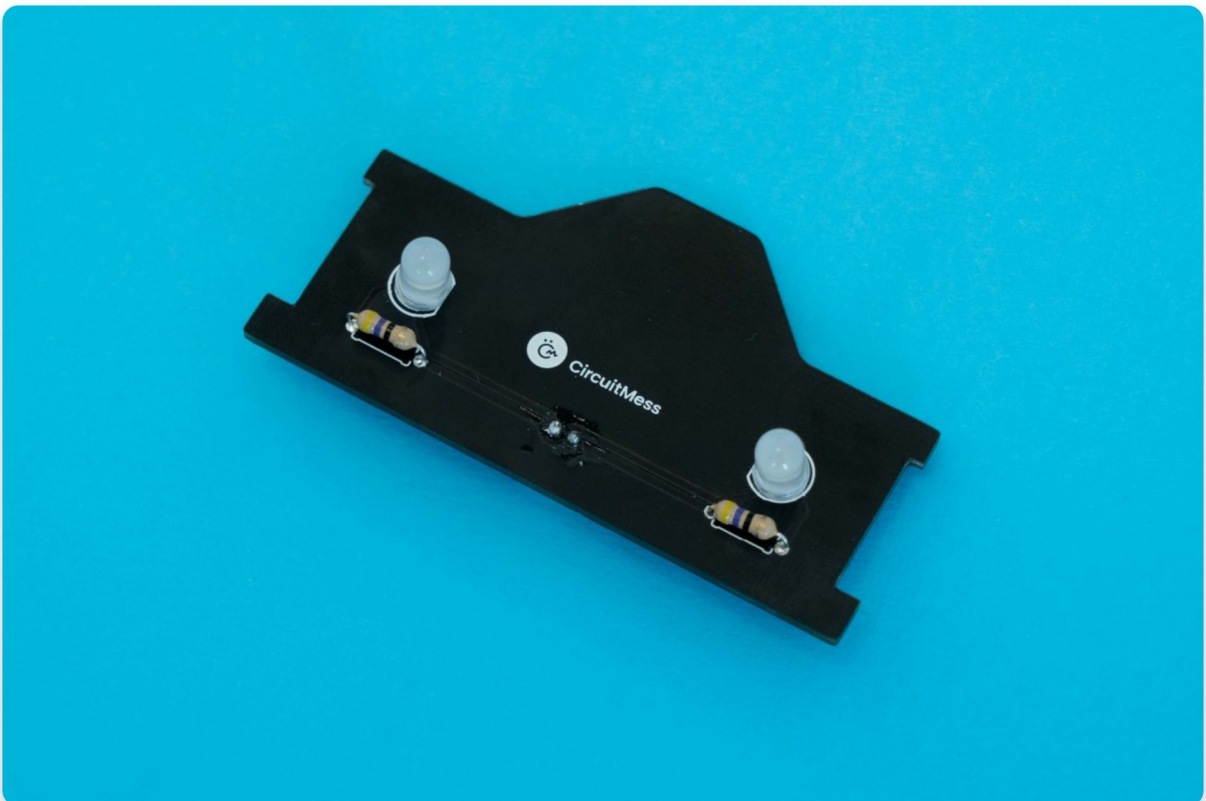
LEDs soldered to the board
