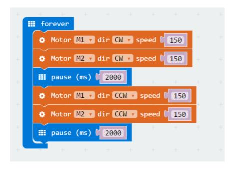
Result: The motor M1 and M2 rotate in positive direction at a speed of 150 for 2 seconds, then
