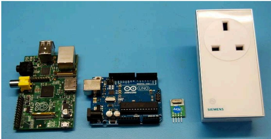
[LightwaveRF](#) (LWRF) is a range of switches, dimmers and other home automation hardware that is widely available in the UK and further afield, sometimes sold under other brands such as Siemens. They are affordable units that are easy to work with.
