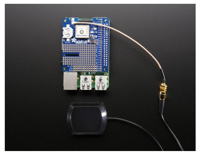
All Ultimate GPS modules have a built in patch antenna - this antenna provides -165 dBm sensitivity and is perfect for many projects. However, if you want to place your project in a box, it might not be possible to have the antenna pointing up, or it might be in a metal shield, or you may need more sensitivity. In these cases, <u>you may want to use an external active antenna.</u> (http://adafru.it/960)
