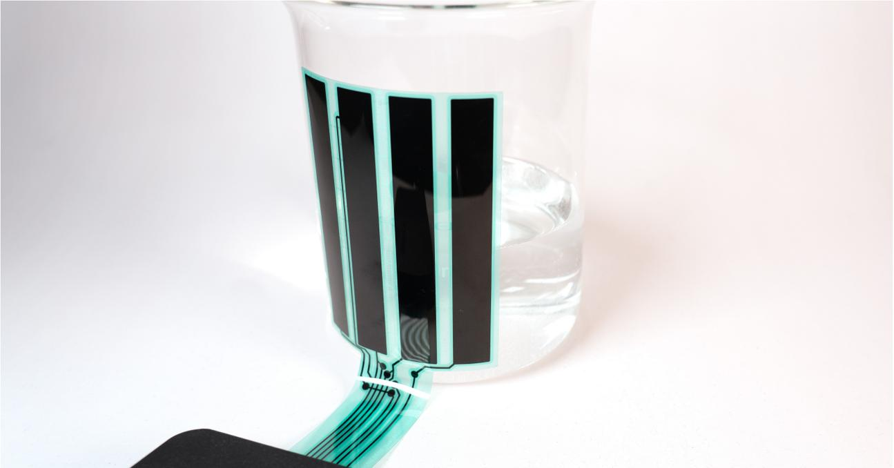
The Trent Evaluation Kit allows you to explore LAIER's Trent technology and test the Trent Sensor against your use cases. It contains the Trent Evaluation Board and LAIER's capacitive Trent Sensors.
