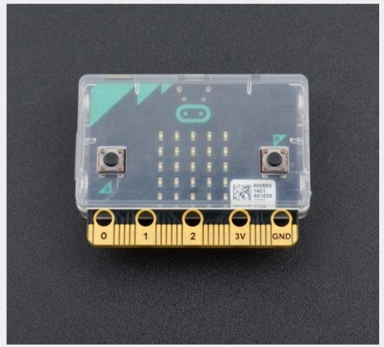
The enclosure has LEGO interface on the back. With LEGO interface, you can build lots of creative projects. It is a perfect combination between micro:bit and LEGO!
