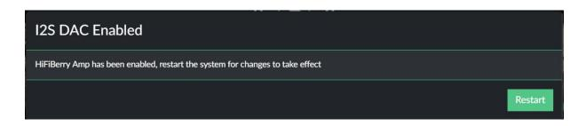
7)In this restart process, "Volumio" hotpot will turn off for a moment. Sometimes your mobile phone or Tablet or PC will automatic connect to other. You need to set back to 'Volumio' hotpot. After restart you can see the main page of Volumio.
