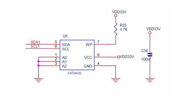
It connected to the same IIC port with AMP you need to solder the IC and Confirm IIC slave devices. If you a novice of Raspberry Pi, We really wouldn't advise do that.
