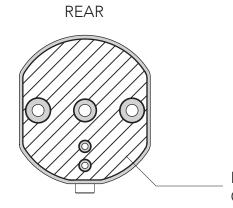
EXPOSED COPPER ELECTRODE CONNECTION ON REAR.
