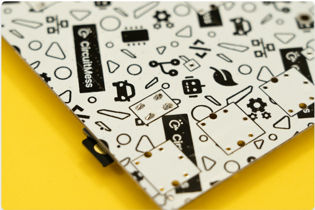
The first pushbutton is soldered to the board
