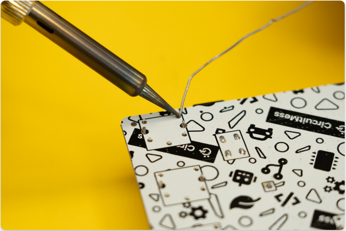
Solder the first pin of the rotary encoder
