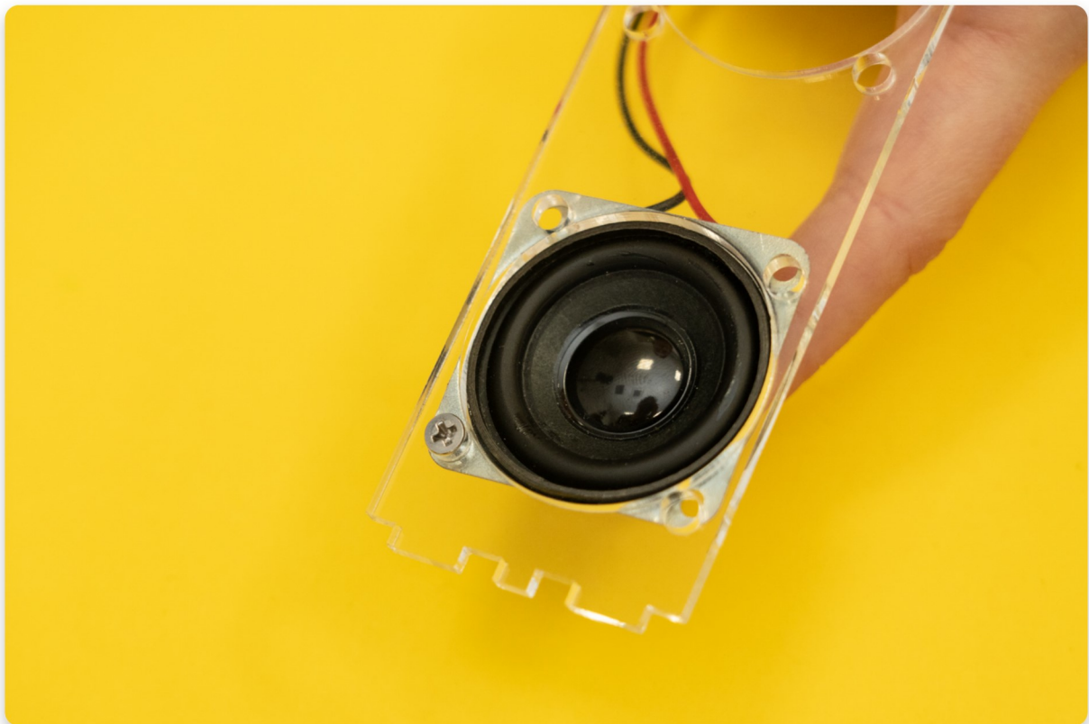
Place the speaker from the bottom of the casing layer and insert the metal bolt from the upper side.
