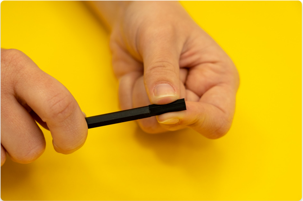
Tighten the black nylon spacer
