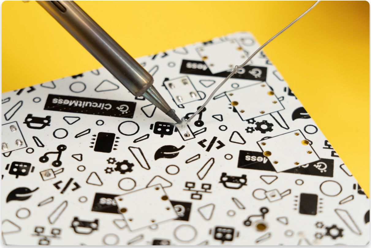
Soldering the two pins
