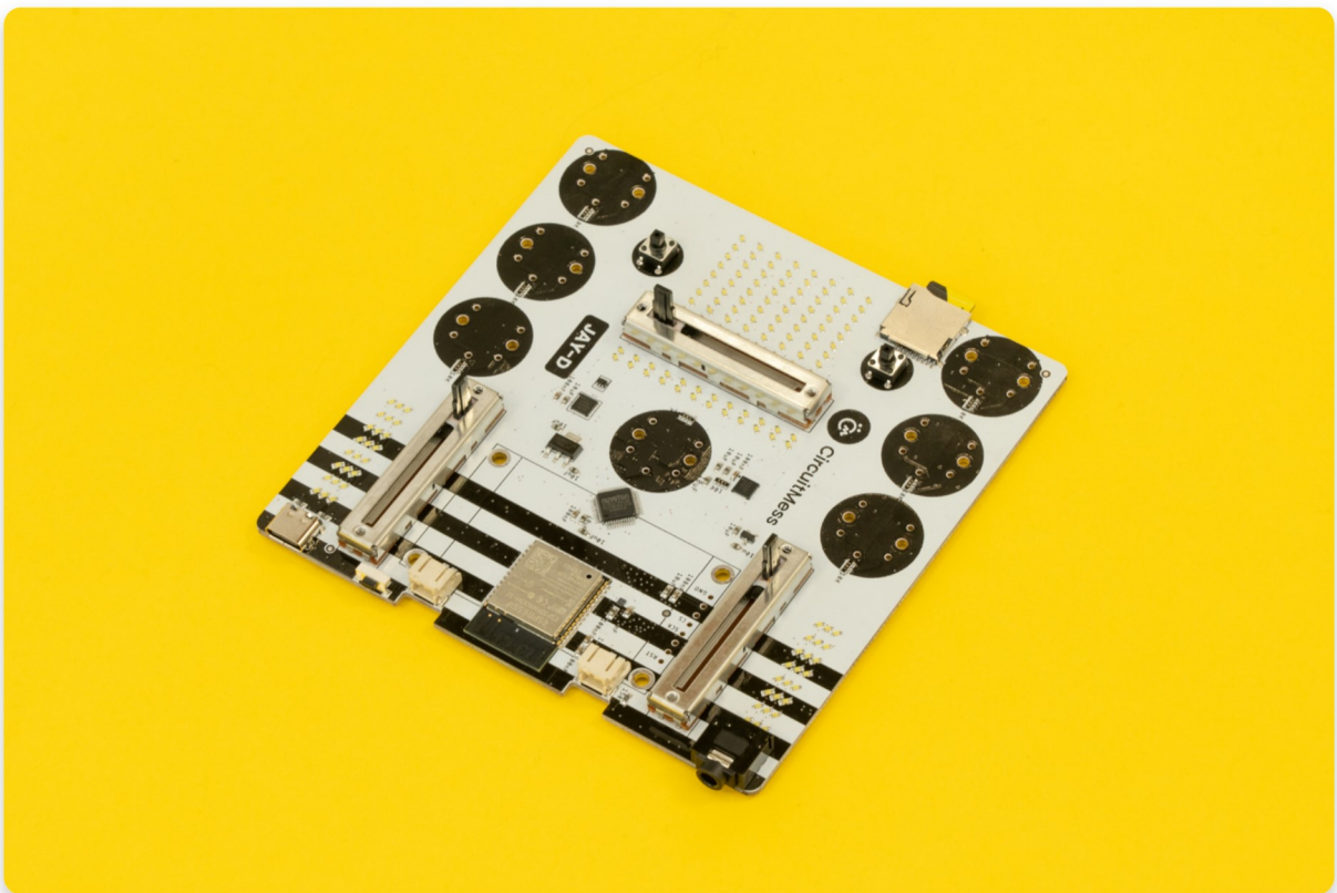
Sliders soldered to the board from the front
