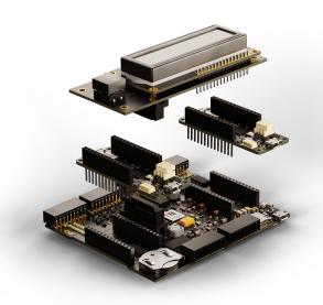
Example of a typical application for a solution including LCD Display and two Arduino MKR 1300 boards.
