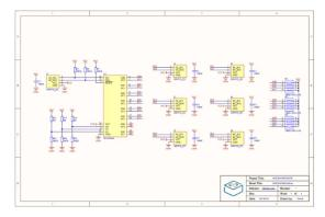
Referring to the schematic diagram and the TCA9548A data sheet, it can be seen that the Unit can modify the I2C address of the device by controlling the level combination of the A0  $\sim$  A2 pins. (Default address is 0x70)
