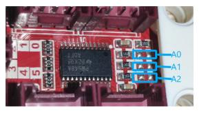
After soldering a 0 ohm resistor, the corresponding pin will change from low to high, and the pin level combination and its corresponding I2C address are shown in the table below.
