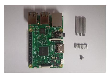
Orientate your Pi to match the above picture and secure the 1" M/F stand offs in the bottom-left, bottom-right and top-right corners using the 1/4" F/F stand offs.
