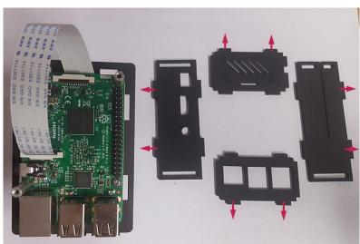
Next thing to do is attach the side acrylic plates. Make sure you have each of the 4 camera box walls in the correct orientation. The edges marked with an arrow should be facing up, opposite side slotting into the bottom plate.
