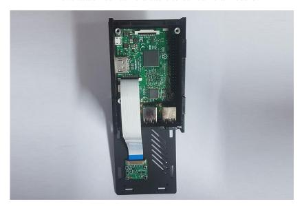
Finally secure the top plate into position using the 1/4" black screws.
