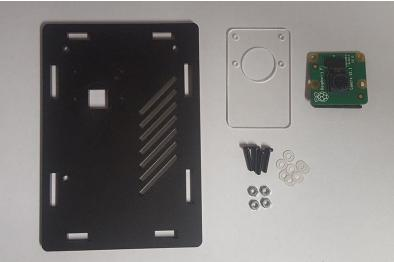
Now we need to attach our camera modle to the front plate. Start by placing the thin clear acrylic plate into position and insert a M2 x 10mm screw into each corner mounting hole.
