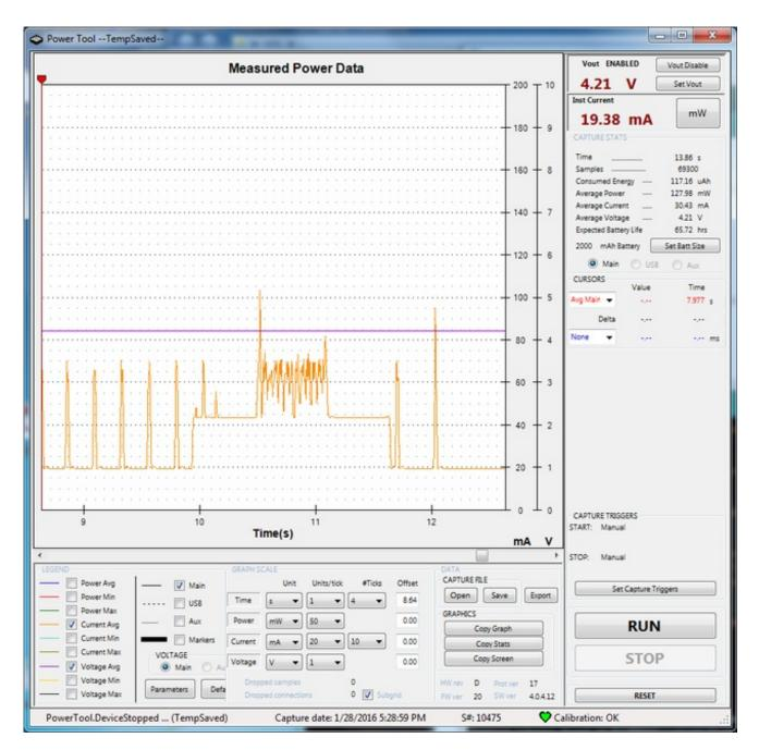
Note that the quiescent current drops from 40mA to 20mA and of that 20mA, about ~12mA is the ATmega32u4. Like we said, the best way to really reduce power for long-term usage is to completely turn off the module with KEY
