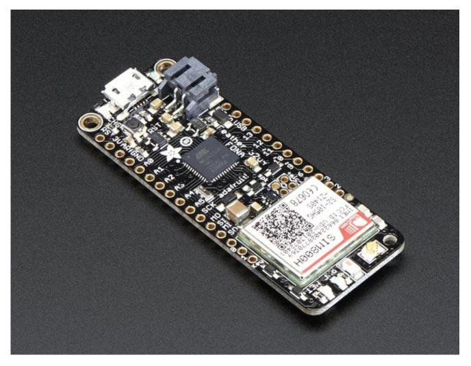
At the Feather 32u4's heart is at ATmega32u4 clocked at 8 MHz and at 3.3V logic, a chip setup we've had tons of experience with as <u>it's the same as the Flora (http://adafru.it/dVI)</u>. This chip has 32K of flash and 2K of RAM, with built in USB so not only does it have a USB-to-Serial program & debug capability built in with no need for an FTDI-like chip, it can
