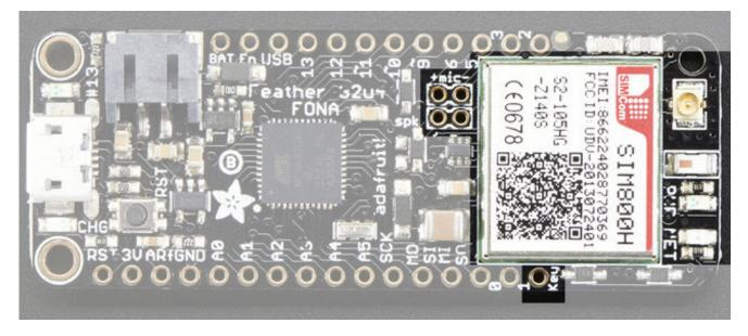
Now to the fun part, the cellular module. There's a few pins that are used to control the module. It uses SoftwareSerial to communicate with the microcoller
