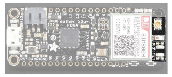
All the way to the right we have the cellular-only connection parts. Up top is a standard uFL connector, you attach your GSM antenna here
