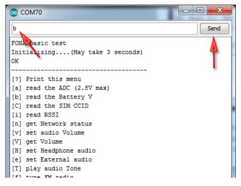
You'll see a print-out of the battery voltage in mV, so in this case its 3.726V
