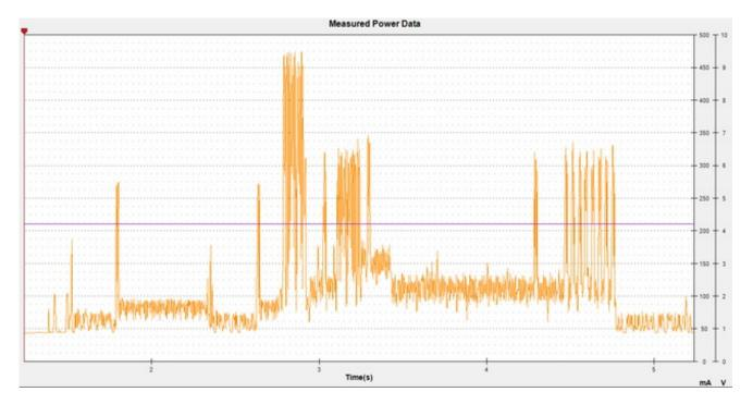
You can put the FONA into sleep mode (with the**AT+CSCLK** command) which will drop the current draw but keep the cellular connection open so you can still receive an SMS and/or wakeup quickly.
