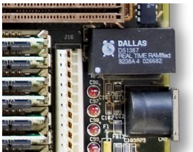
This image shows a computer motherboard with a Real Time Clock called the DS1387 ( http://adafruit.it/aX0 ). There's a lithium battery in there which is why it's so big.
