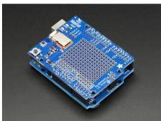
If you are using the Bluefruit LE Shield then you have an SPI-connected NRF51822 module. You can use this with Atmega328 (Arduino UNO or compatible), ATmega32u4 (Arduino Leonardo, compatible) or ATSAMD21 (Arduino Zero, compatible) and possibly others.
