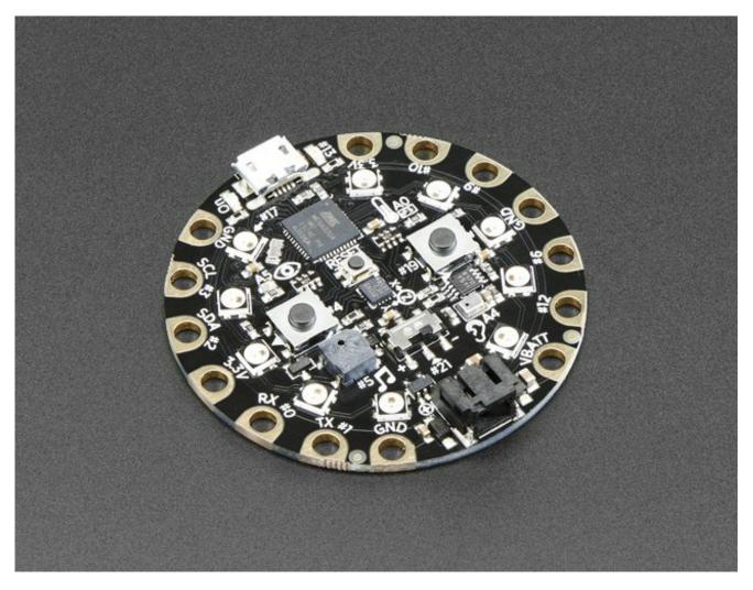
Circuit Playground has built-in USB support. Built in USB means you plug it in to program it, it just shows up - all you need is a Micro-B USB cable, no additional purchases are needed! With the new 1.6.4+ Arduino IDE, it takes only a few seconds to add support (http://adafru.it/nb4). The Circuit Playground has USB HID support, so it can act like
