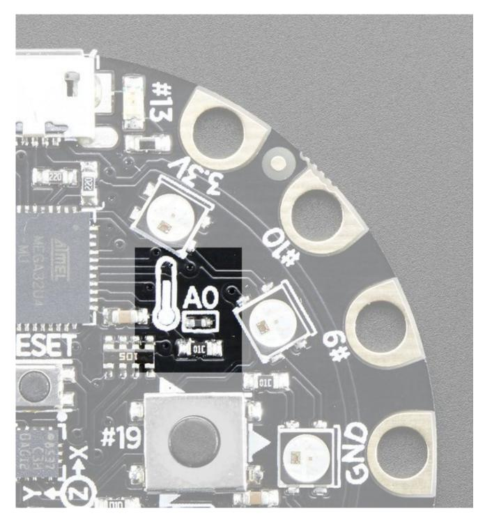
There is an NTC thermistor (Murata NCP15XH103F03RC) that we use for temperature sensing. While it isn't an all-in-one temperature sensor, with linear output, it's easy to calculate the temperature based on the analog voltage on analog pin **#A0**. There's a 10K resistor connected to it as a pull down.
