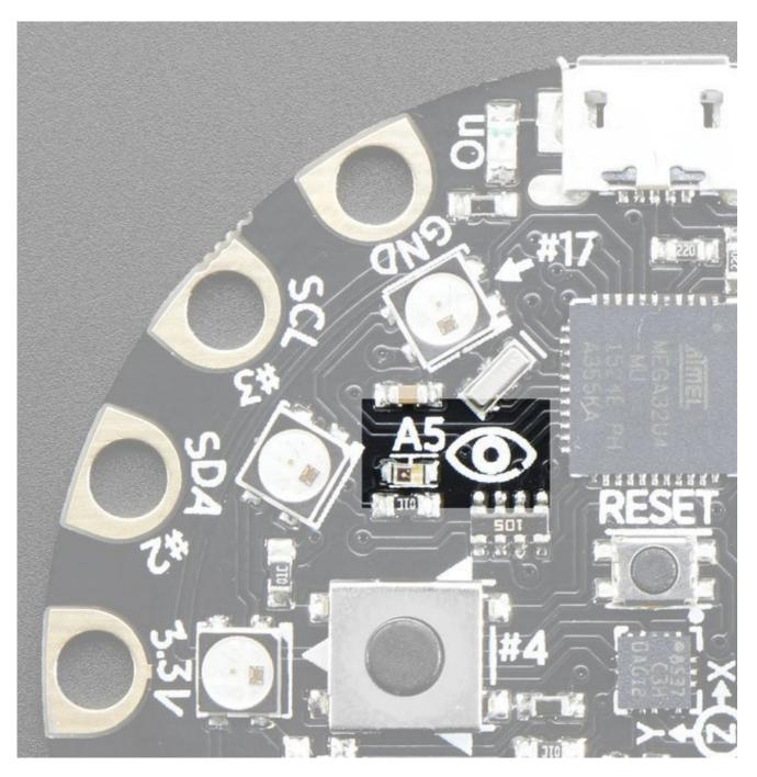
There is an analog light sensor, <u>part number ALS-PT19</u> (http://adafru.it/n8F), in the top left part of the board. This can be used to detect ambient light, with similar spectral response to the human eye.
