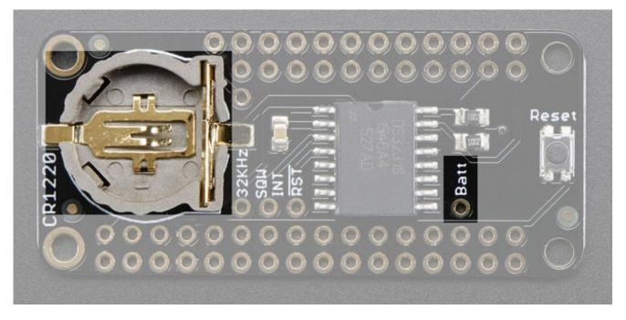
A CR1220 battery holder is on-board for long term RTC timekeeping. A new CR1220 should be able to power the DS3231 for at least 5 years. If you want to use that battery for powering something else (maybe a GPS module or a very low power BLE beacon?) you can connect to the **BATT** breakout on the very right.
