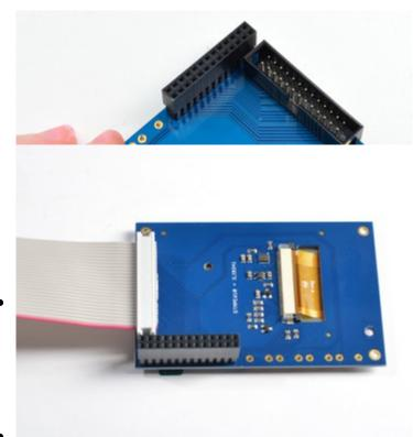
product to include an IDC socket so it's easier to add a cobbler. Both will work, though!
