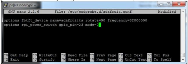
To make it active immediately run sudo modprobe rpi\_power\_switch
