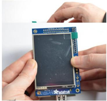
Once you have the screen so it is definitely not touching the header, you can gently press on the sides to secure the tape.
