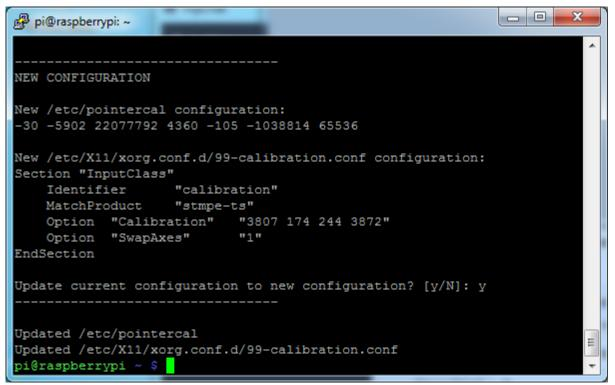
Try using this default calibration script to easily calibrate your touchscreen display. Note that the calibration values might not be exactly right for your display, but they should be close enough for most needs. If you need the most accurate touchscreen calibration, follow the steps in the next section to manually calibrate the touchscreen.
