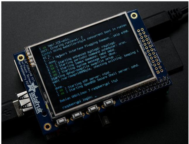
One fun thing you can do with the display is have it as your main console instead of the HDMI/TV output. Even though it is small, with a good font you can get 20 x 40 of text. For more details, check out <a href="https://github.com/notro/fbtft/wiki/Boot-console">https://github.com/notro/fbtft/wiki/Boot-console</a> (http://adafru.it/cXQ)
