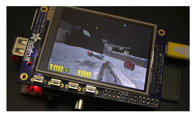
**The Ideal:** Adafruit's PiTFT displays are razor sharp. Whereas small composite screens on the Raspberry Pi usually require some video scaling (resulting in blurriness), PiTFT uses the GPIO header, digitally controlled pixel-by-pixel for a rock steady image. Though not a *lot* of pixels, it works great for retro gaming (and the display neatly stacks above the board, no side protuberances for video cables).
