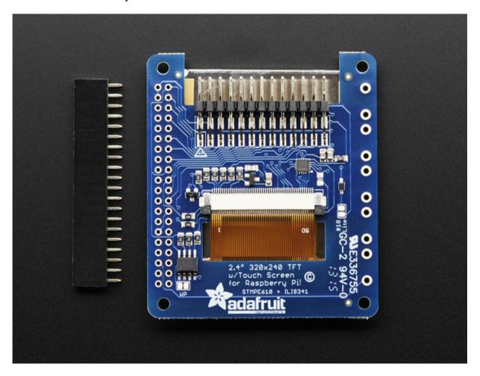
Check also on the back that the TFT is attached and that the flex connector is seated into the onboard FPC socket.
