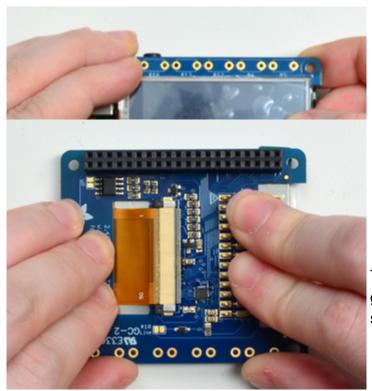
Turn the board over and press gently on the back to get the TFT stuck-on well!
