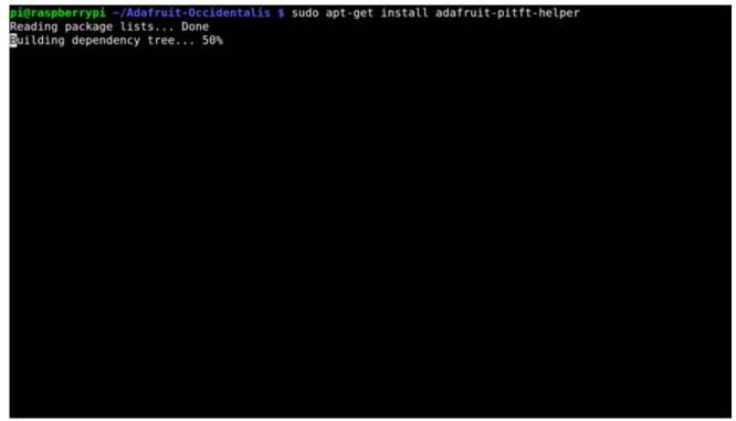
It's normal for the Pi to pause at this step for up to 20 minutes, theres a lot of kernel software to replace
