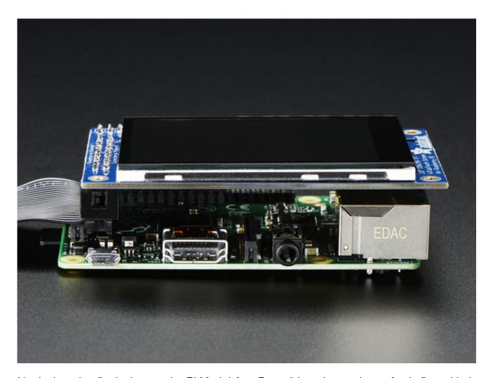
It's designed to fit nicely onto the Pi Model A or B rev 2 but also works perfectly fine with the Model B+ as long as you don't mind the PCB overhangs the USB ports by 5mm, see the photos above. Model B rev 1 have an older layout for the I2C pins and won't be able to use the touch screen
