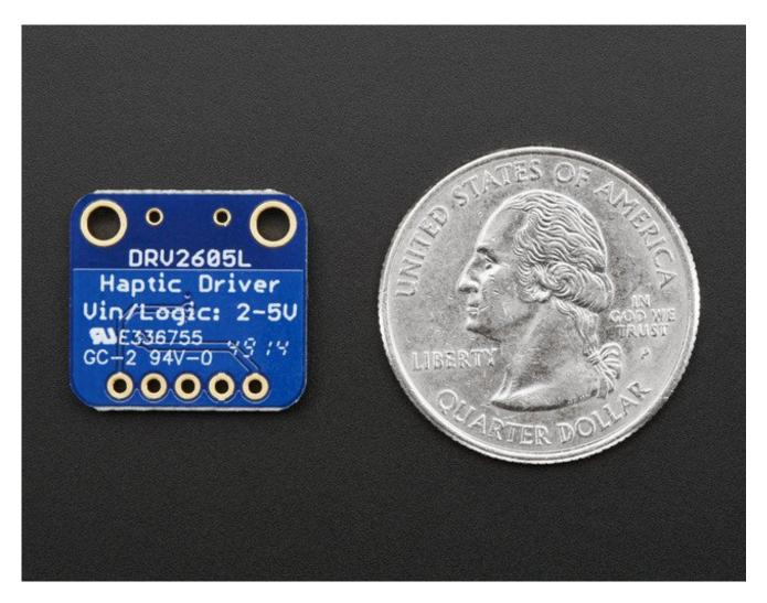
According to the product page, it can be used with both LRA (Linear Resonance Actuator) and ERM (Eccentric Rotating Mass) type motors <u>but we have only used it with our little vibration pancake ERM.</u> (http://adafru.it/dDc)
