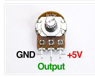
Potentiometers don't care which outer leg is ground or +V, but the choice does affect which direction has increasing output.
