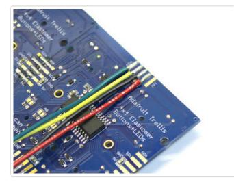
Try pointing the wires "inward" rather than off the edge of the board. This makes it easier to fit in the case.
