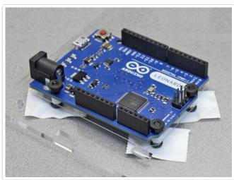
Now turn the base over, remove the tape (if used) and <u>gently</u> tighten the three screws with a small screwdriver.
