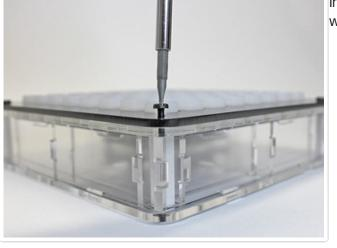
Install four corner screws through both top waffles and into the standoffs.
