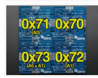
When setting the board addresses (by bridging the solder points on the back), use the values shown here.
