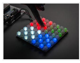
Four *Trellises* are combined to make a single large **8x8 matrix** for UNTZtrument. The HELLA UNTZtrument has *eight* Trellises in a 16x8 matrix!
