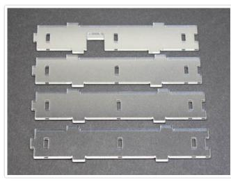
The four side pieces are *almost* identical... except for one which has a notch for the Arduino's USB port. Install this side first. Align the bottom tabs with the slots in the base and tilt it up into place. If the USB port is covered, you've got it backwards — turn it around and try again.
