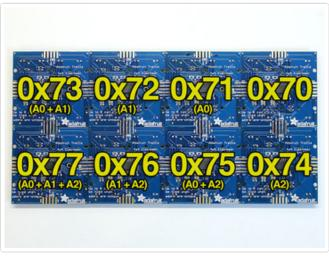
Here's the address map for the HELLA UNTZtrument.
