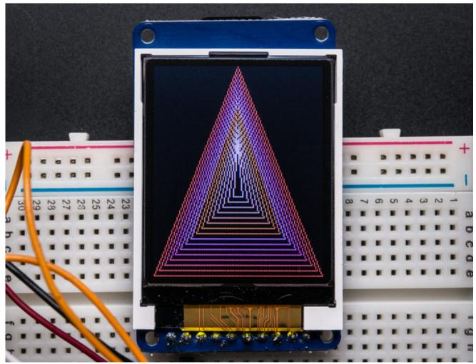
Once uploaded, the Arduino should perform all the test display procedures! If you're not seeing anything - first check if you have the backlight on, if the backlight is not lit something is wrong with the power/backlight wiring. If the backlight is lit but you see nothing on the display make sure you're using our suggested wiring.
