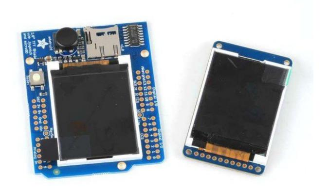
The 1.8" display has 128x160 color pixels. Unlike the low cost "Nokia 6110" and similar LCD displays, which are CSTN type and thus have poor color and slow refresh, this display is a true TFT! The TFT driver (ST7735R) can display full 18-bit color (262,144 shades!). And the LCD will always come with the same driver chip so there's no worries that your code will not work from one to the other.
