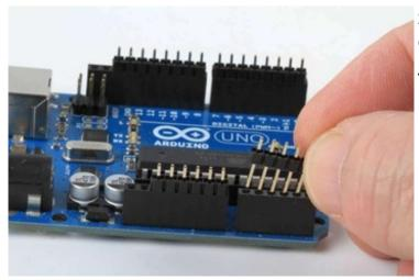
2 unused pins on the end closest the USB and DC power jacks.
