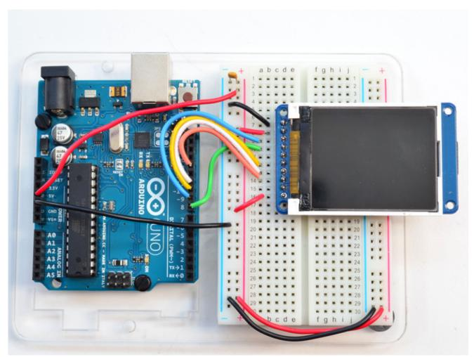
Once you are sure that the TFT is wired correctly, add the two wires for talking to the SD card. Connect **CARD\_CS** (the unconnected pin in the middle) to digital pin4 (you can change this later to any pin you want). Connect **MISO** (second from the right) to the Arduino's hardware SPI **MISO** pin. For Classic arduinos, this is pin 12. For Mega's this is pin 50. You can't change the **MISO** pin, its fixed in the chip hardware.
