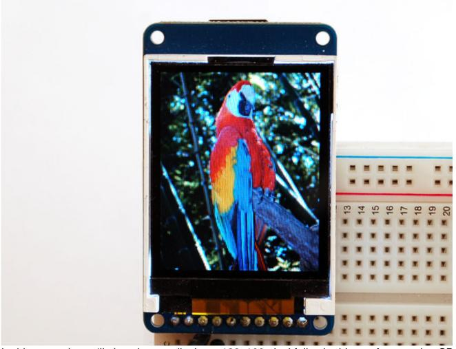
In this example, we'll show how to display a 128x160 pixel full color bitmap from a microSD card.
