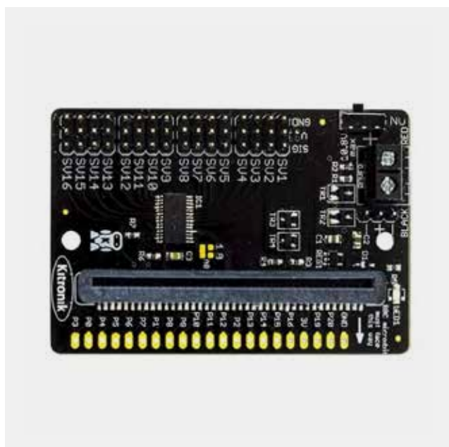
Compact 16 Servo Driver Board for BBC micro:bit SKU: 2048219 MPN: 5694
