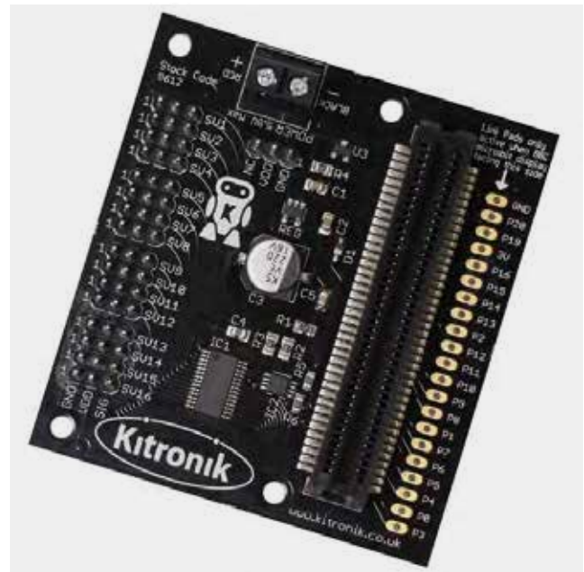
Compact Motor Driver Board for BBC micro:bit SKU: 2048223 MPN: 5698
