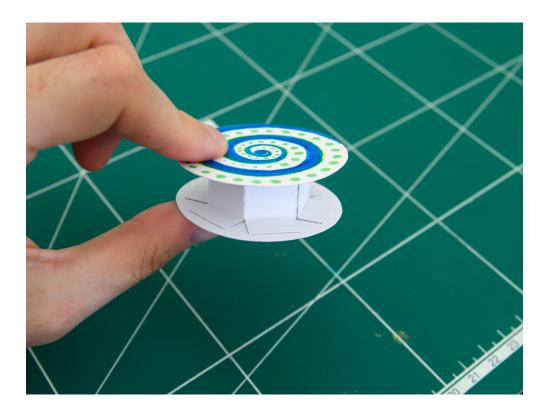
Use the center mark on the drum side to position and tape one of the servo horns to it. It doesn't matter which servo horn you use, but the cross shape it easy to tape because of the long arms.
