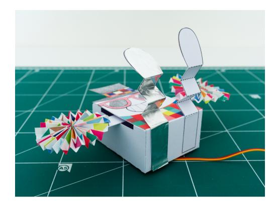
Add another small piece of tin foil or conductive tape at the center-bottom of the body as shown. If you want both legs to be ticklish, make sure that this smaller piece touches the foil on both legs.
