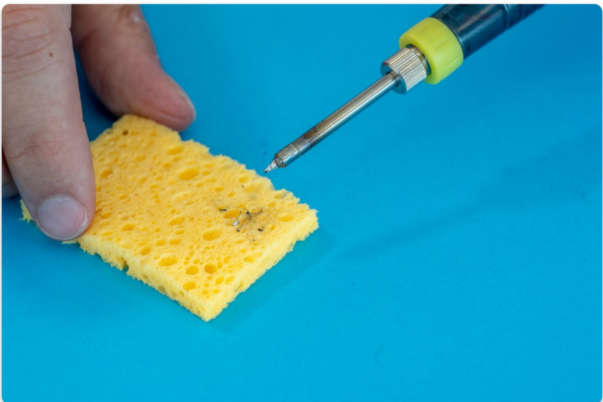
Cleaning the tip of the soldering iron
