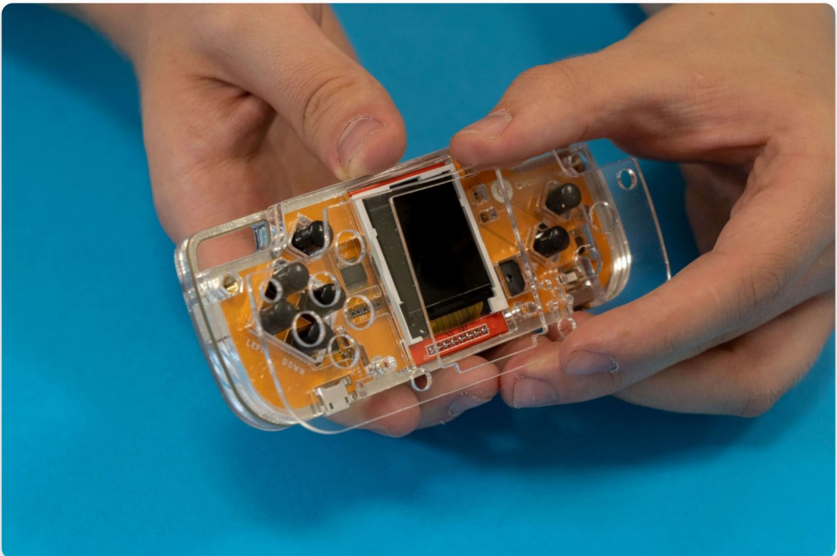
Placing the top layer - the final layer of the "sandwich"
