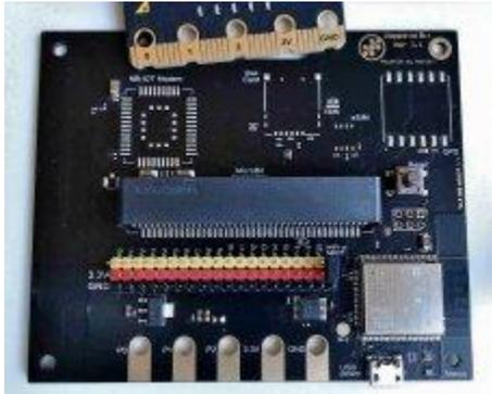
With our basic board, the unequipped soldering places for the SD card, the GPS and the IoT-NB module for the other Wappsto: Bit variants are visible.
