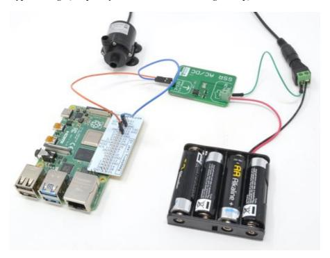
In this screnario, a GPIO pin of the Raspberry Pi is directly used to control the SSR switching a water pump powered from a 4xAA battery pack.
