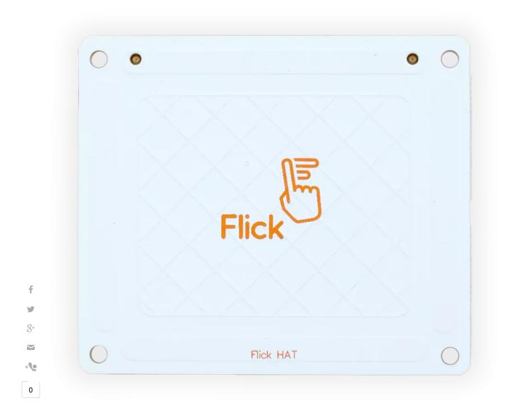
**Step 4** – Place the Flick HAT on top of the Raspberry Pi by gently pushing the female header onto the Raspberry Pi male header.
