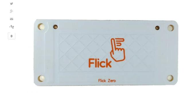
**Step 5** – Screw the last 4 plastic bolts to hold the Flick Zero in place.
