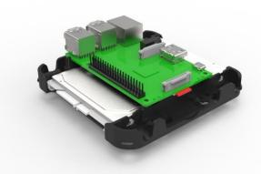
\* Removeable cover to gain access to the SD card
