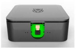
The "logo" cover can be removed easily to gain access to the SD Card / Camera PCB.
