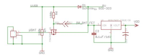
Espruino's power circuitry is as above. When USB is connected the device is powered through a Schottky diode with 0.3v voltage drop. However when USB is disconnected then Espruino can be powered from a battery with no voltage drop. This is done by turning on the PFET Q1.
