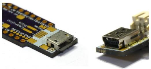
On the rear of the Pico Board under the while block of silkscreen, there are pads for connectors. Espruino rev 1v3 has both Micro and Mini USB, but Espruino rev 1v4 only has Mini USB (due to potential issues with Apple's USB extension leads).
