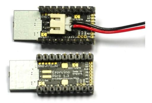
Espruino Pico contains the circuitry needed to power itself from a battery without the voltage drop of a diode. This means that it will run off of normal 3.7v LiPo batteries (or any voltage up to 16v).
