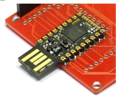
The Pico is designed to be easy to include in your designs. The 0.1" pins are easy to fit in to sockets, and castellated edges mean that unpinned Picos can easily be surface-mounted directly to a PCB.
