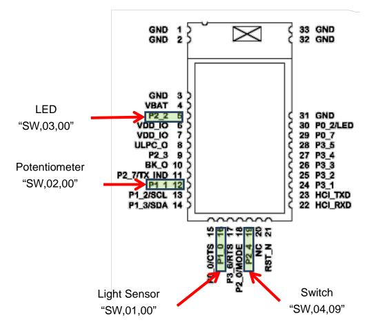
Figure 16: RN4870 Pins used by Sensor Board Interface
