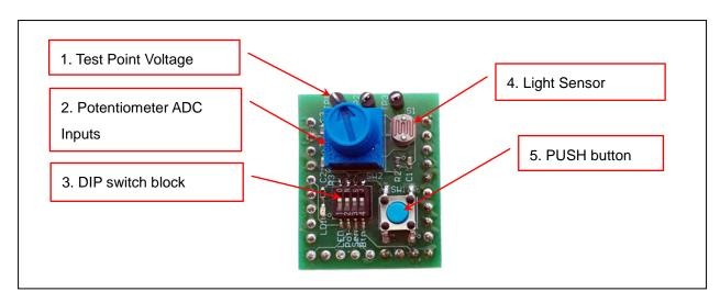
Figure 4: Sensor Board Interfaces
