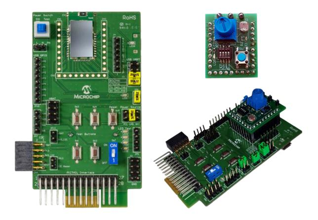
Figure 1: RN4870-SNSR (includes PICTail and Sensor Board)
