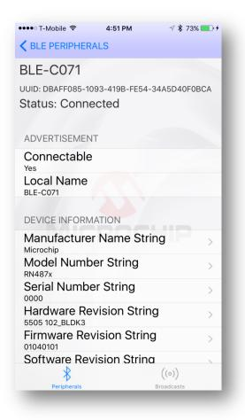
Fig 11: GATT Service when Connected
