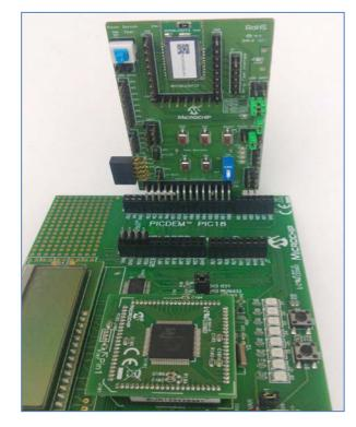
Figure 30: PIC18 Explorer Board with RN4870 PICtail Plus
