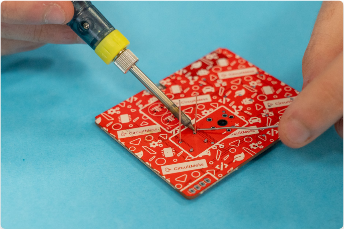
Solder the second resistor
