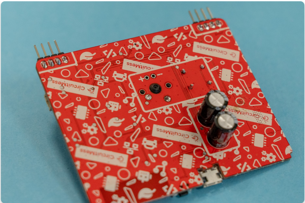
The button is now soldered
