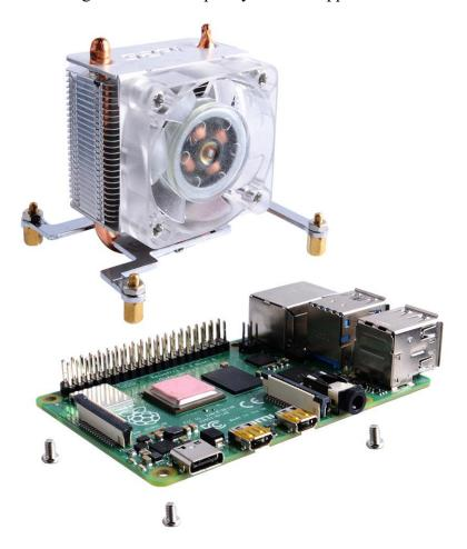
5. Fixed Acrylic protection holder to Raspberry Pi with M2.5 screws.
