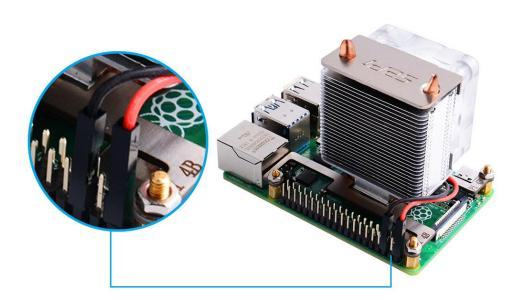
7. While the Ice Tower's fan is massively loud, it can get a little irritating. There's a quick solution: moving the red power cable from a 5V pin on the Raspberry Pi's GPIO header to the 3V3 pin instead. This can reduce both the fan speed, noise, and the brightness of the LED light, at the cost of it pushing less air through the heatsink stack.
