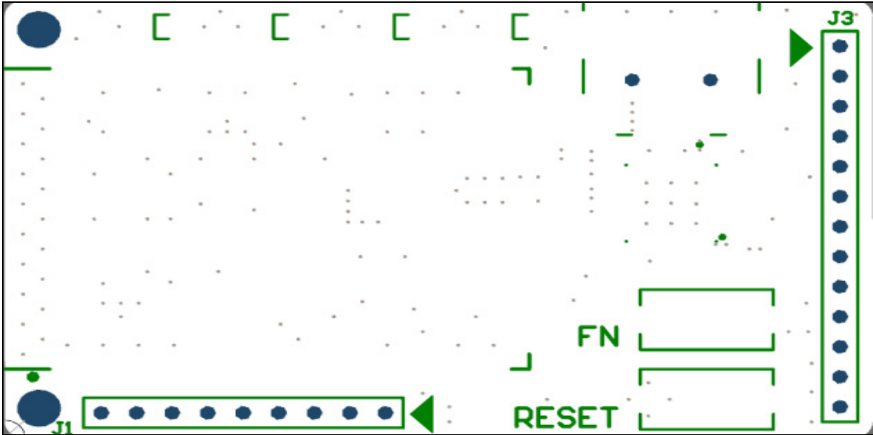
FIGURE A-3: RN131 EVALUATION BOARD TOP SILKSCREEN
