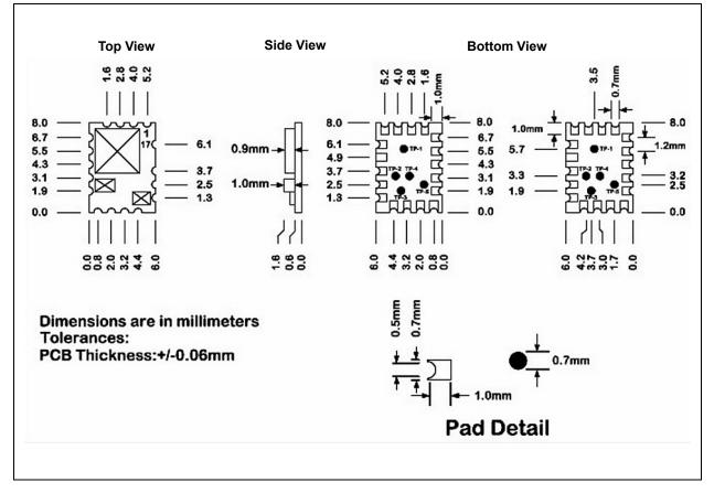
FIGURE 4-10: RN4871U MODULE DIMENSIONS
