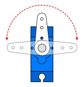
The **Standard Micro Servo** (also called a Positional Micro Servo) can only rotate 180° — half a circle. You can control the exact position it goes to by programming the angle. You can't control the speed.
