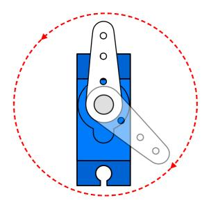
The Continuous Rotation Micro Servo can rotate 360° — a full circle. It can go around continuously in either direction. But the trade off is that you can't control the exact position it goes to — all you can do is program the speed and the direction it spins in.
