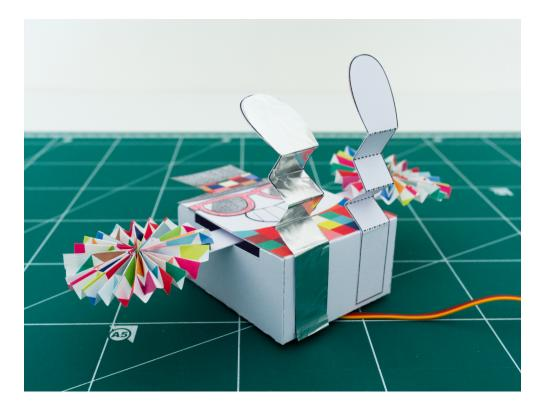
Add another small piece of tin foil or conductive tape at the center-bottom of the body as shown. If you want both legs to be ticklish, make sure that this smaller piece touches the foil on both legs.
