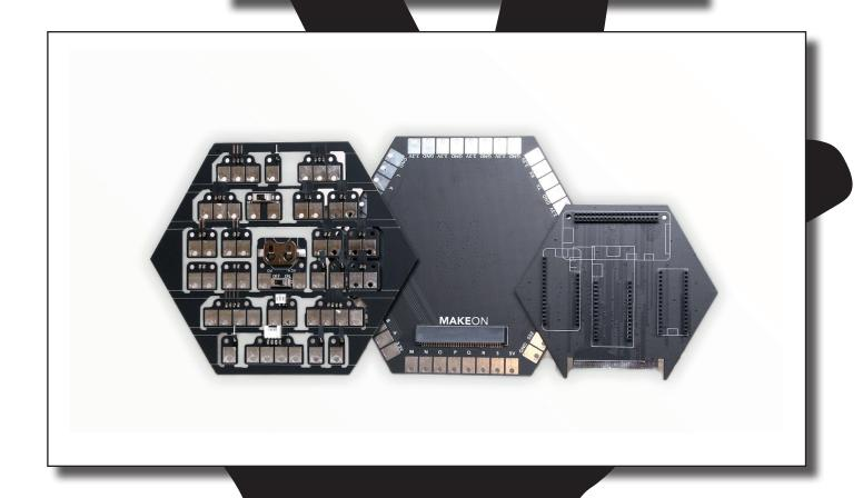
» This all in one set is the ultimate breakout set. Connect components by clip, clamp, tape, paint, rivet, solder, sew and snaps. The size of the "pads" allow clear connections to be made less fiddly. The card reader mounting is soldered on both sides making it durable and low profile at the same time. It is an excellent choice for low profile requirements, such as in tight places, like wearables, walls and more!
