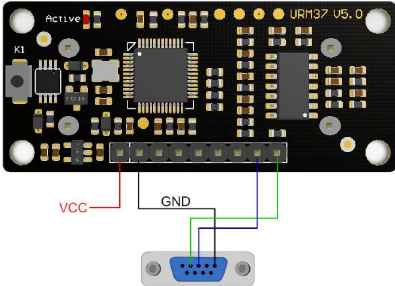
Power on the sensor, read the blink of the LED(active) to get the serial level(see above), wire according to the above picture. After this, you can use our "URMV3.2HelpMate (<https://www.dfrobot.com/image/data/SEN0001/URMV3.2HelpMate.rar>)" to test the module.
