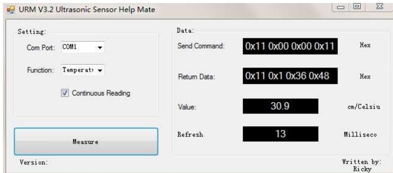
The usage of the software is very simple: ensure that there is no other software on the computer occupying the serial port, and then run Mate.exe, select the COM Port, and choose the parameter
