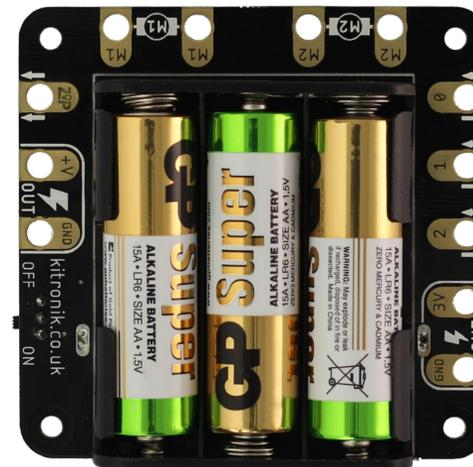
The Klip Motor Driver requires 3 x AA batteries to provide power to the connected BBC micro:bit and any extra attached devices. These are shown inserted in the correct orientation in the image to the left.
