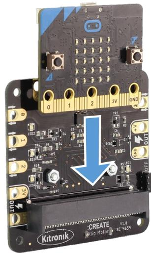
The BBC micro:bit needs to be firmly inserted into the edge connector with the BBC micro:bit LEDs visible to the user.
