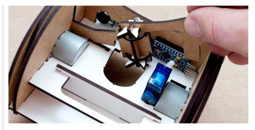
Then drop the wide end down so it fits into the slot and rests on top of the  ${\sf servo}$
