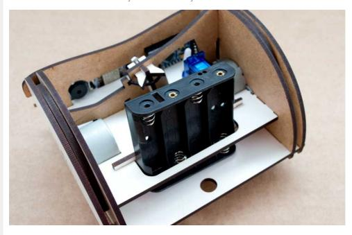
On the underside, plug it into the power socket on the main controller board. You may need to wind it around some other cables slightly to keep it nice and neat. Don't wind it too tightly otherwise it can be hard to get it out when you chenge the batteries.
