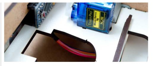
On the underside, wind the servo wire around the hooks you wound the stepper wires around and plug the wire in to the 3 pin servo pins on the main controller board. Make sure you align the yellow wire with the "Y" mark on the board.
