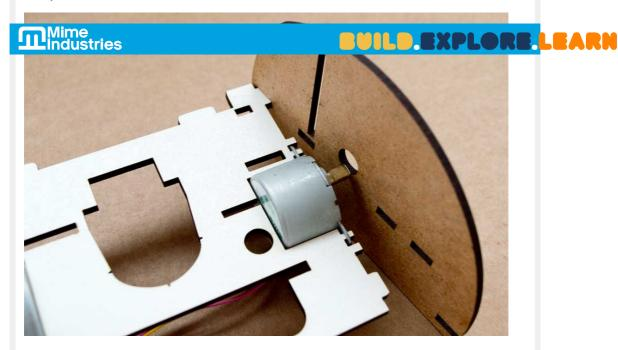
Once it is in place, push the other wheel (panel 2 or 3) on to the stepper motor which will hold the second side piece in place
