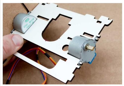
Hook the right side (panel 4) on to the front of the base and push it on fully.
